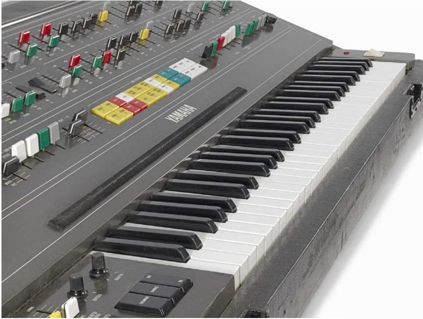
FIGURE 4. Close-up view of the Yamaha CS-80's ribbon controller, located below the Yamaha logo. The material of the Yamaha ribbon's contact surface is flocked felt, giving it a velvety, more tactile sensation as compared to the smooth, satiny metal feel of the Moog ribbon. Photo © Deutsches Museum, Archives, Munich, CD 75304, reproduced with permission.
