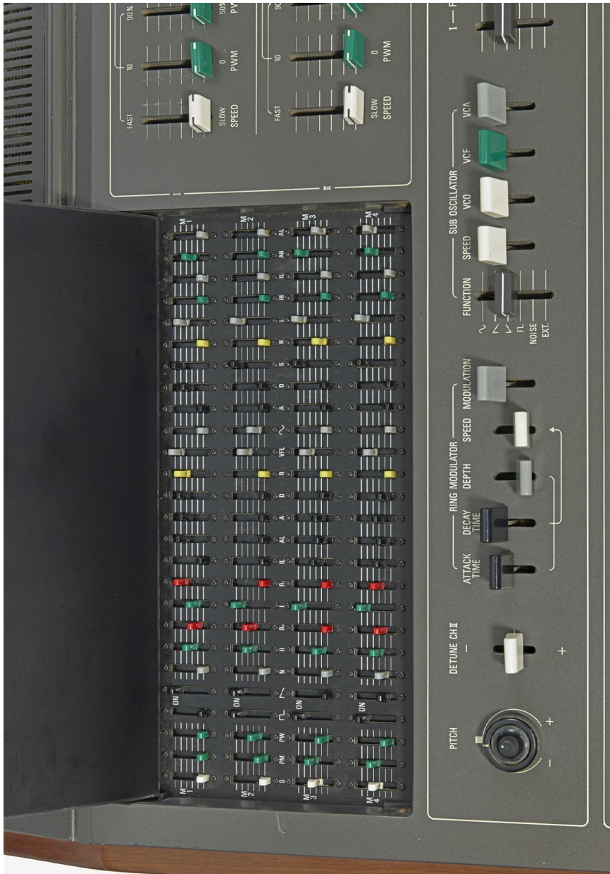
FIGURE 2. Close-up view of the Yamaha CS-80's programmable memory bank, located inside the cover, under the block diagram. Photo © Deutsches Museum, Archives, Munich, CD 75305, reproduced with permission.
